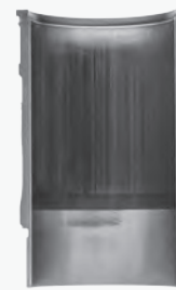
Severely Scuffed Liner
