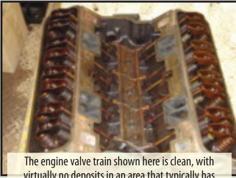
The inside of the valve cover is very clean with almost no deposits.
